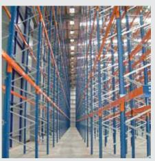
Upright slots are positioned in 75mm increments, giving you greater flexibility when choosing beam levels.
