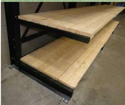
**Cantilever racking - safe and neat storage, especially suited for long products**
