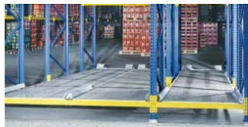
*To avoid damage in everyday use, entry guides and roller protectors are an extremely robust design*
